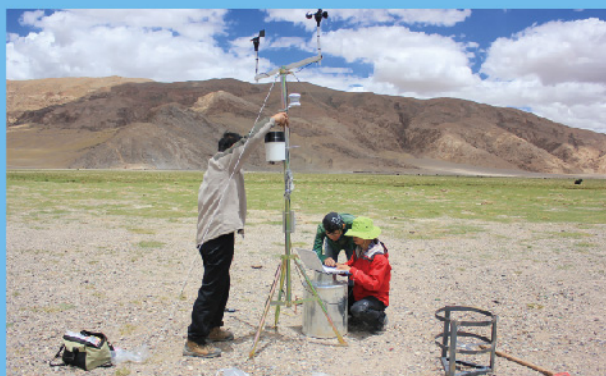
AWS configuration and testing in the field
