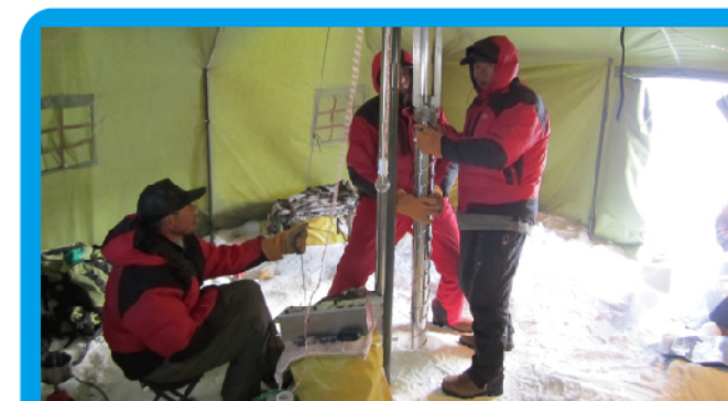
Chinese scientists retrieving ice cores with an independently developed ice drill
